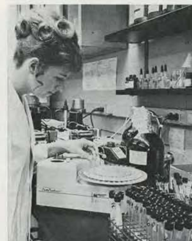
Autoanalyzers test samples of body fluids for constituents, increasing accuracy and shortening the time required. Analyzers detect and measure blood lipids that may accumulate and contribute to heart disease.
