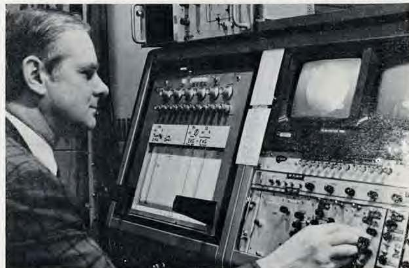
Mr. Whitehouse adjusts the position of the videodensitometer on the TV screen during a heart catheterization procedure. Closed circuit television is used to determine the ejection fraction of the left ventricle.
