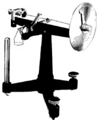
Central Scientific Co. (CENCO) du Nouy Precision Direct Reading Model Tensiometer
